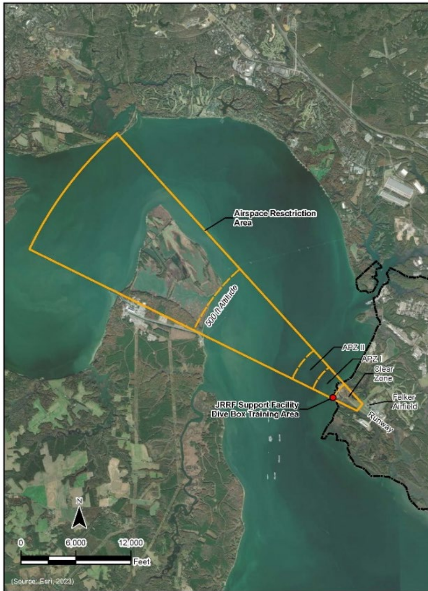
Figure 9 - Height Restriction Diagram for Felker Airfield
